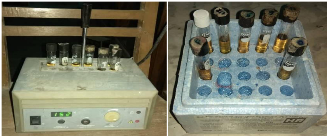
Fig 6: Sample preparation for the calculation of COD.
