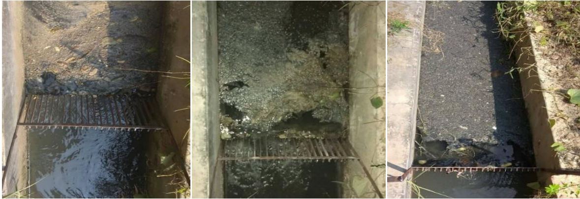
Fig 5: Observation of the drain after 1, 12 and 24 hours of installing the bar screen.
