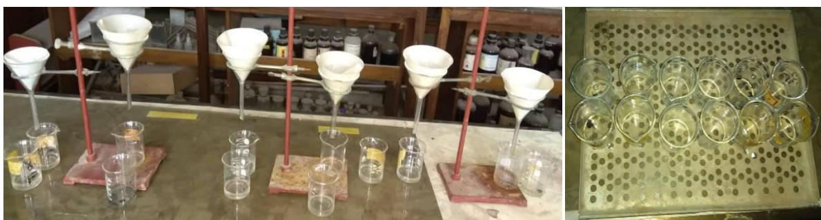
Fig 7: Sample preparation for suspended solids and total dissolved solids.
